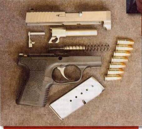
The Kahr CM9 fieldstrips as seen using only a simple tool, but reading the instruction manual first is a must. Disassembly is seldom necessary.
